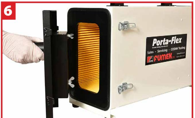
6 Refit the front cover and then reattach the four toggle fasteners to secure it in place. The extractor is now ready for use.
