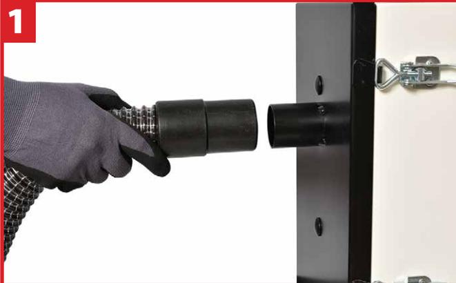
Place the Porta-Flex on a sturdy, level surface and connect the 2.5m extraction hose to the intake port. This is located on the front of the unit.
