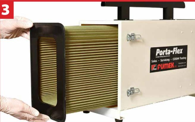
3 Slowly withdraw the old filter horizontally and place in a plastic bag and then seal the bag with tape. **NB. Old filters must be disposed in accordance with Local Authority Guidelines.**
