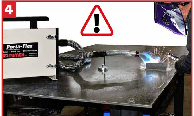
Position magnetic nozzle so that fumes/gases are drawn AWAY from the operator. Ensure that hose is not kinked or trapped. Please refer to certification for capture distance.
