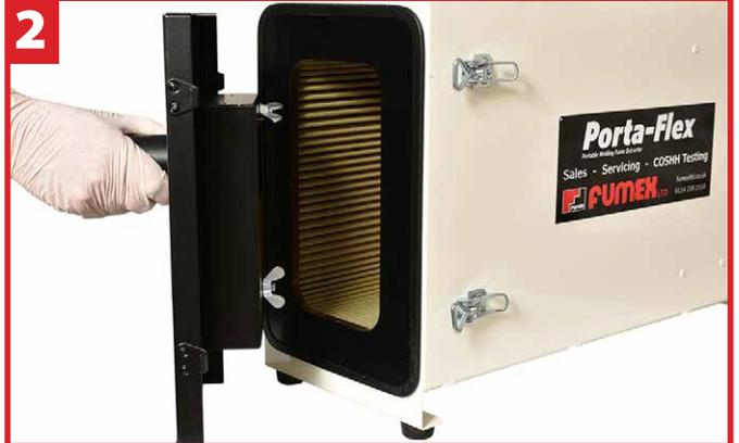
2 Carefully remove the front cover and combined spark trap. Check the spark trap, by removing the two wing nuts and clean if required.
