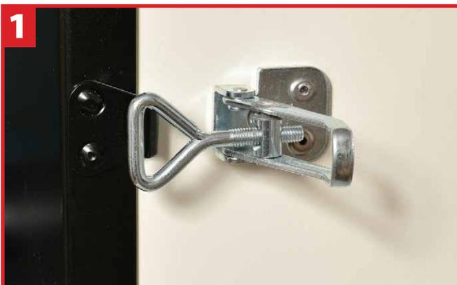
To access the spark trap, release the four toggle fasteners and unhook the front cover.
