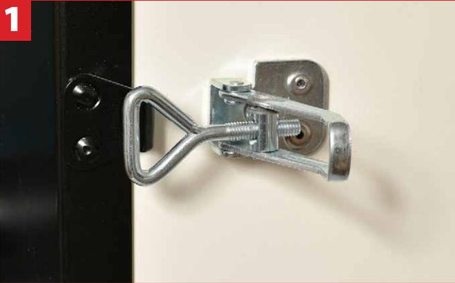
1 To access the cartridge filter, release the four toggle fasteners and unhook the front cover.
