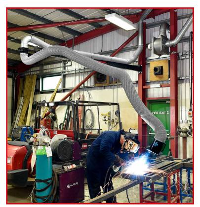
The Flexi Crane Arm is designed to extract welding fumes and grinding dust at source. It's ideal for use in general engineering, fabrication and automotive/plant use.
